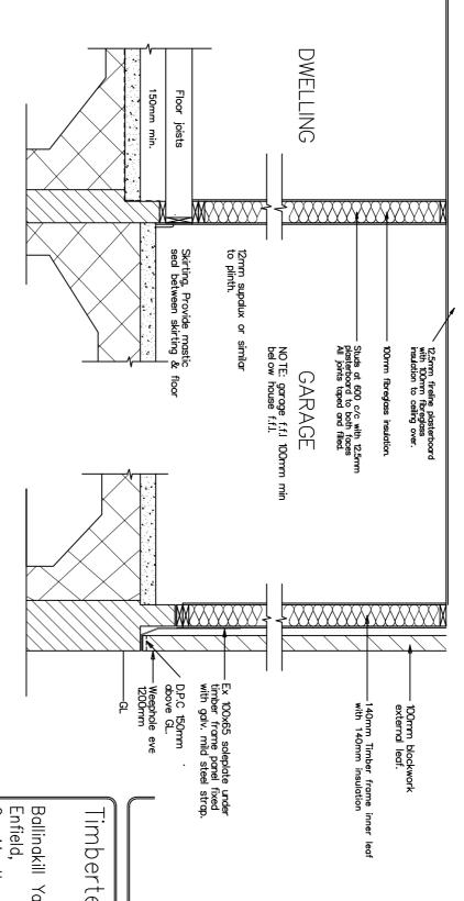
Junction of Suspended Timber Floor to Garage Concrete Floor
